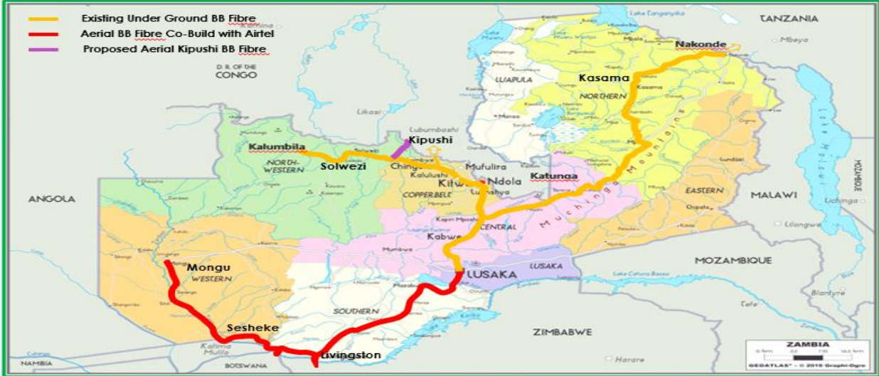
Figure 29: MTN Zambia Aerial and Underground Backbone Fibre Network
